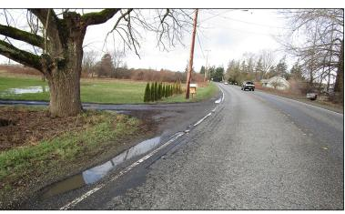
This project consists of widening of the roadway to City standard, including 5' wide shoulders, new sidewalks, crosswalks, streetlights, and bus pullouts.
