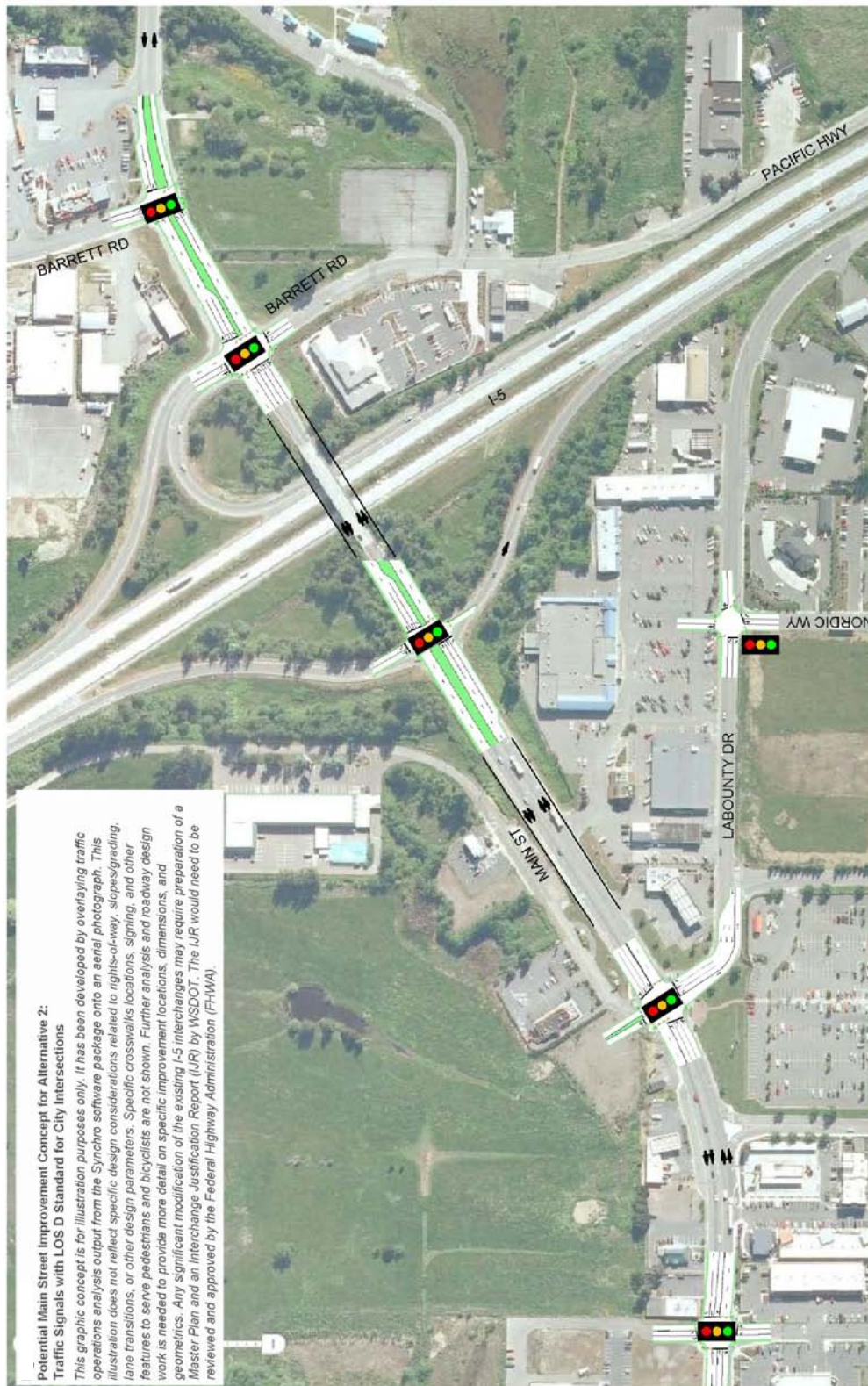
Figure 2-4 Potential Main Street Improvement Concept for the Preferred Alternative – Traffic Signals with LOS D Standard for City Intersections
