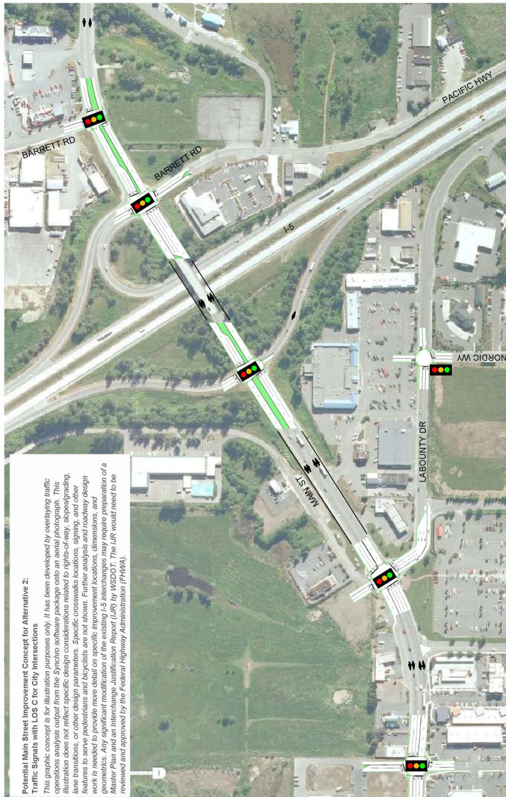
Figure 2-2 Potential Main Street Improvement Concept for the Preferred Alternative – Traffic Signals with LOS C Standard for City Intersections
