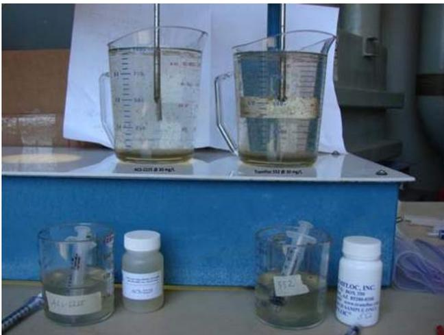
Jar Test 3, ACS-2225 and Tramfloc 552 both at 30 mg/L
