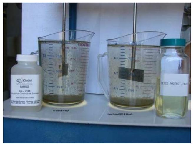
Jar Test 3: CC-2135 and Protect 7025 both at 30 mg/L
