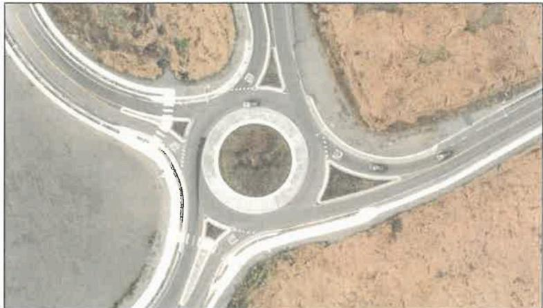
This project upgrades the compact roundabout at I-5 northbound Portal Way into a full size roundabout with slip lanes. Pedestrian, bike friendly improvements are included.
