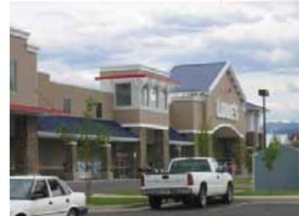
**Gable** means a triangular wall section at the end of a pitched roof, bounded by the two roof slopes.
